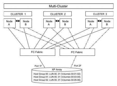
Within the Storage Area Network (SAN), the clusters may be homogeneous (all the same operating system) or they may be heterogeneous (mixed operating systems). How you configure LUN Security and fabric zoning depends on the operating system mix and the SAN configuration.
